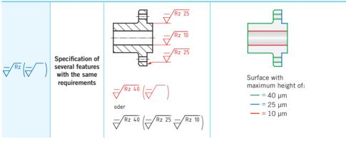
Collective indications for identical surface requirements must be placed close to the title block of the drawing.
