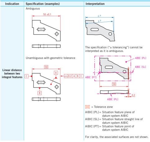
The toleranced, extracted surface must be within the tolerance zone (linear, width 0.2 mm). The tolerance zone is constrained in terms of orientation and location in relation to the situation features of the AIBIC datum system.
